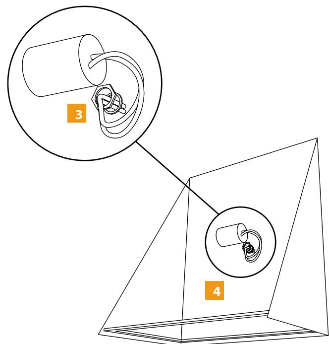
**4** Now feed wires through mounting hole through back of fixture and thru nipple that is mounted to electrical box.
